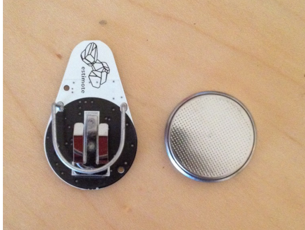
Figure 3. Tear down of an iBeacon (Estimote version) [9].
