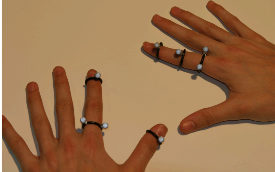
Figure 18, Markers to track finger gestures [Grossman et al. 2004] .
