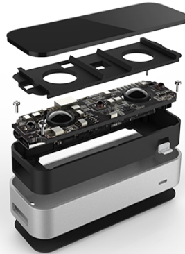
Figure 13, Exploded view of the Leap Motion Controller [2014].
