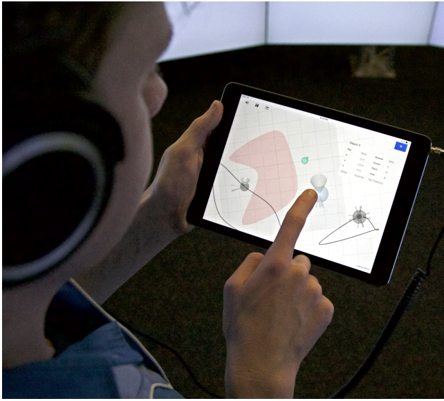
Figure 2: A user exploring the augmented reality in CAVE system, while using a mobile device to edit the 3D sonic virtual reality he is hearing through headphones. The user is controlling the position of an object in lateral-view mode.
